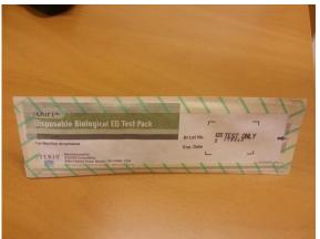
*Figure 9: Tyvek layer of blister package for entering and exit of VHP vapor*
