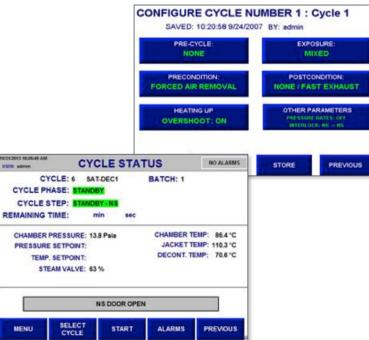
STERIS is now offering the new PanelView Plus 6 display which replaces the older Allen Bradley PanelView series. The new series offers several improvements over the older displays which are now discontinued and no longer serviceable.
