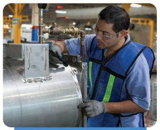
Each pressure vessel is individually inspected and hydro pressure tested.
