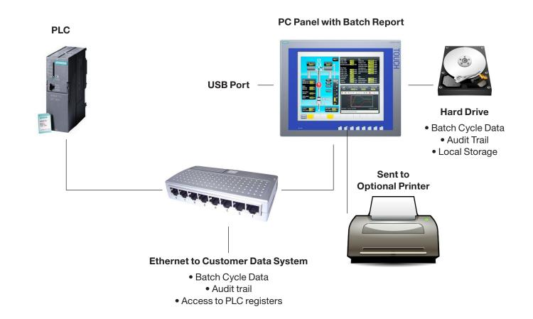
Upgraded Siemens® control package provides 21 CFR Part 11 and EU Annex 11 capability with data archiving and enhanced batch reporting.
