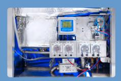
Up to four chemical injection pumps are included to handle most soil conditions. The conductivity monitoring system tracks detergent injection and final rinse water quality.
