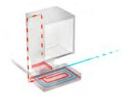
The effluent heat recovery system allows heat to be recovered from the hot water being drained to preheat cold water used for the next cycle. The system also greatly reduces the need to use cold water for drain cooling.
