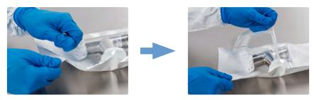
A laboratory simulation was conducted, demonstrating the process of wrapping and unwrapping equipment using BPS products is faster and generates significantly fewer particles when compared to using cellulose based materials. The difference is greatest when the equipment and/or operations are complex.
