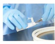
Product contact surfaces of a filling needle assembly are protected using a BPS small drawstring bag.
