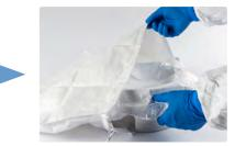
Covered equipment is placed into a BPS bag as secondary protection during sterilization, storage, and transport to the manufacturing area.
