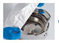
The product contact surface on the stopper bowl is protected using a fitted, elasticized BPS cover.
