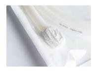
Filling needle and tubing assembly with ends covered are placed within a BPS polyolefin/film sterilization pouch.
