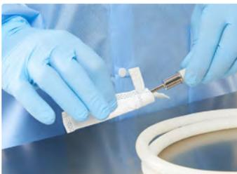
Product contact surfaces of a filling needle assembly are protected using a BPS small drawstring bag.
