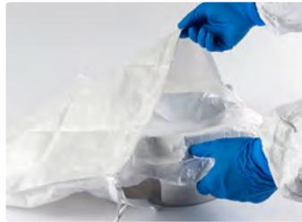
Covered equipment is placed into a BPS bag as secondary protection during sterilization, storage, and transport to the manufacturing area.
