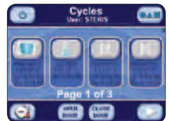
Password protected, supervisor adjustable cycle parameters
