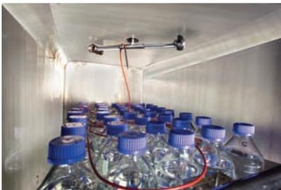
Air ejectors in chamber for SAMX cycle
