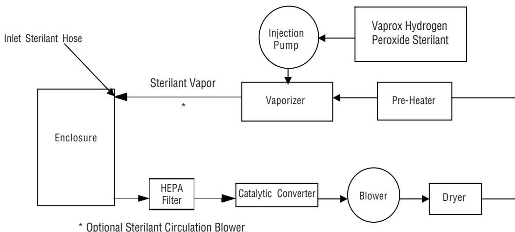
Figure 1 - Typical Closed-Loop Process Diagram
